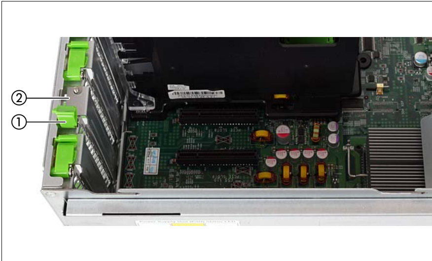
Figure 34: Inserting the new expansion card
